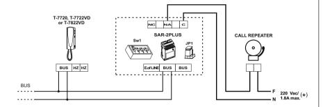
(\*)The neutral supply of the additional call repeater will be wired through the relay contacts SAR-2Plus, the maximum current for the additional call repeater will be 1.8A.
