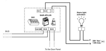
(\*)The neutral supply of the stairs light will be wired through the relay contacts SAR-2Plus, the maximum current for the additional element will be 1.8A.
