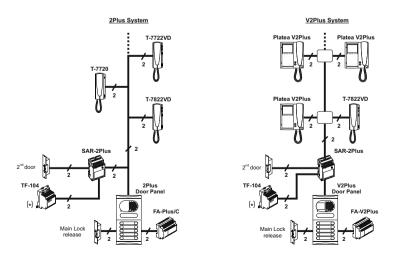
(\*) Lock release supply arrives through the contacts of SAR-2Plus relay.
