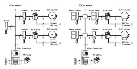
(\*) The neutral supply of the additional call repeater will be wired through the relay contacts SAR-2Plus.
