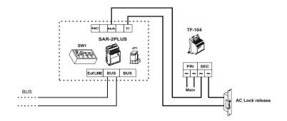
onfiguration of the digital relay unit.
