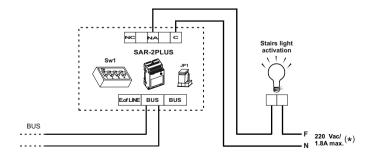
(\*)The neutral supply of the stairs light will be wired through the relay contacts SAR-2Plus, the maximum current for the additional element will be 1.8A.
