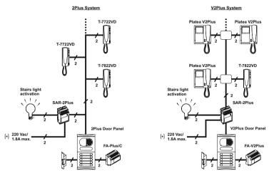
(\*) The neutral supply of the stairs light will be wired through the relay contacts SAR-2Plus.
